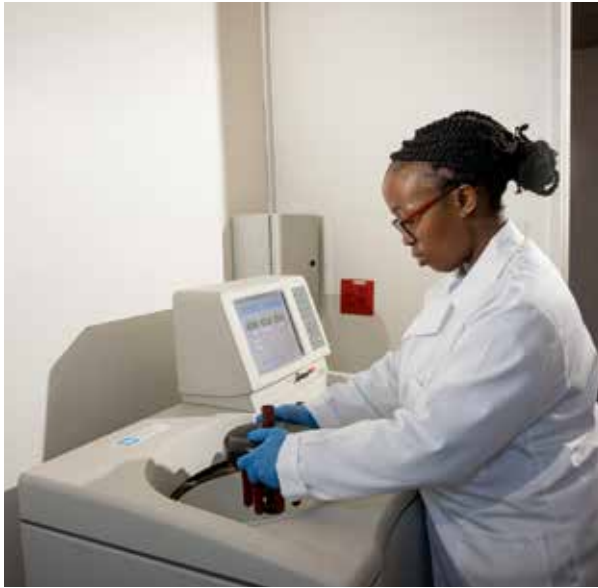
Nozipho Mlotshwa using a ultracentrifuge to purify viral particles on vaccine development.
